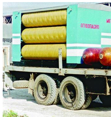
Figure 2. Equipment for mobile CNG stations: a) mobile methane refueling, b) CNG cylinders for CNG stations, c) methane transporter.
