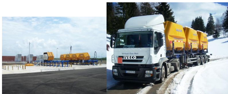
Figure 6. "Virtual pipe" technology equipment by Galileo company.
