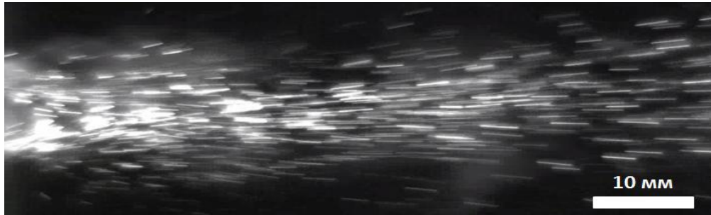
Figure 2. Video image of two-phase plasma flow with zirconia particles tracks. Nitrogen flow rate 45 slpm, arc current 200 A, arc voltage 190 V, powder feedrate 2 kg/h. Exposure time 40 mks.
