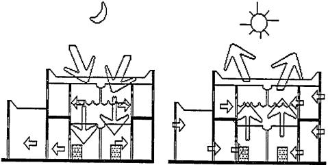
Figure 2.2. Section through the traditional courtyard house explaining (Aleid, 1994)
