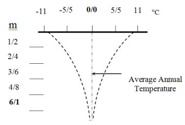
Figure 2.4. Underground annual temperature fluctuations versus depth
