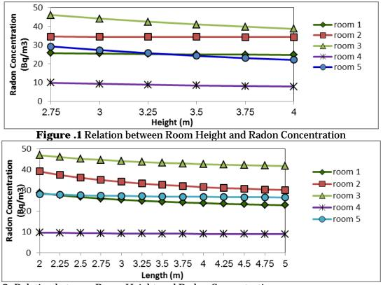
Figure 2. Relation between Room Height and Radon Concentration
