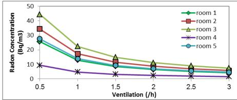
Figure 3. Relation between Ventilation and Radon Concentration
