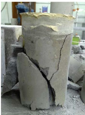
Figure 13: Failure mode of 1000 kg/m<sup>3</sup> density at ambient temperature
