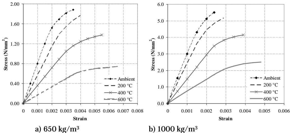
Figure 5: Stress-strain relationships under compression at different temperatures
