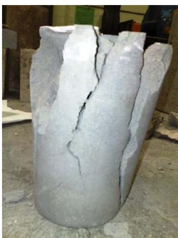
Figure 14: Failure mode of 1000 kg/m<sup>3</sup> density at 400°C
