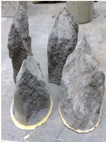
Figure 11: Failure mode of 650 kg/m<sup>3</sup> density at 400°C
