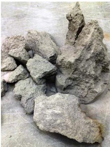
Figure 12: Failure mode of 650 kg/m<sup>3</sup> density at 600°C
