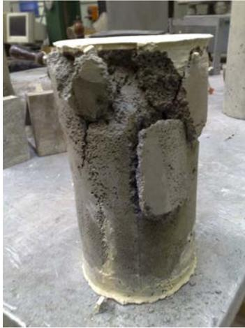
Figure 10: Failure mode of 650 kg/m<sup>3</sup> density at ambient temperature
