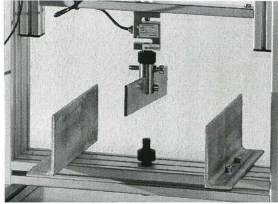
Figure 4: Setup for three point bending strength test
