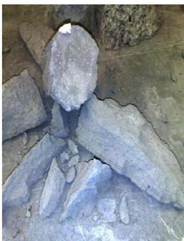
Figure 15: Failure mode of 1000 kg/m<sup>3</sup> density at 600°C
